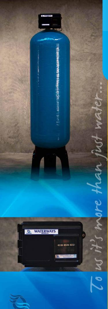
**Product Description:** Mixed bed filters are used for sediment removal over a wide range of flow rates. Due to a much larger surface area and the ability to be backwashed the dirt holding/handling capability of a mixed bed filter is far superior to cartridges. The beds can be made up of different filtering sands and filtration media.
